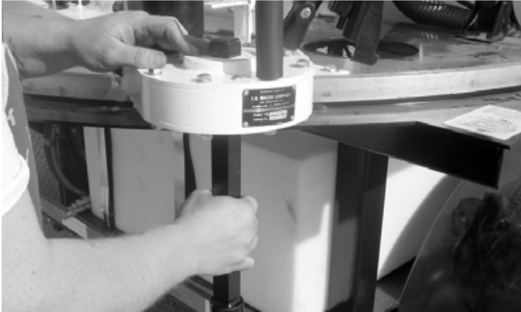
*Figure 3-4. Insert the valve key adapter up through the bottom of the head.*
