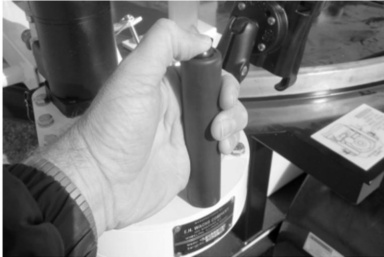
Figure 3-2. Hold down the brake release button to move the ERV-750 arm.
