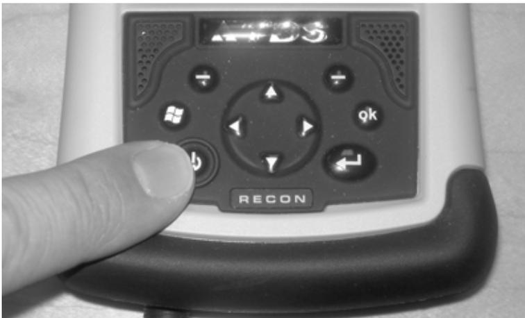
Figure 3-8. Press the power button to turn on the ERV control pendant.
