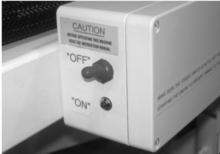
*Figure 1-5. Push the power switch on the control box down to turn on power to the ERV-750.*
